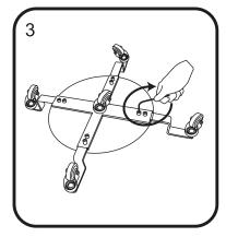
Tighten the frame by using of hexagonal-key.
