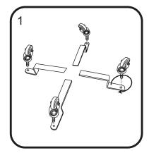
Please screw the wheels onto the bottom side of the frame in clockwise direction, as picture above.
