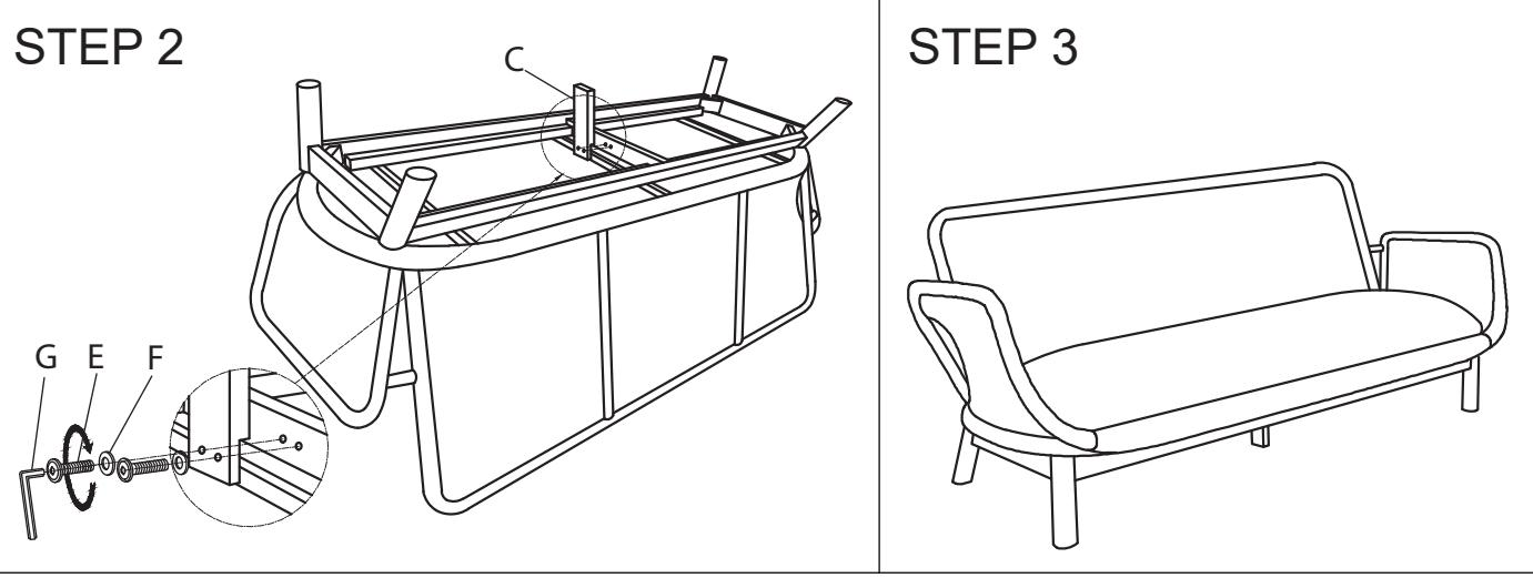
Remark: Be noted, during assembly, we recommend only to tighten all screws with 80% fastening, when having all screws in correct position, and tightened to 80% - then OK to tighten to 100%, to avoid any distortion, bendings.
