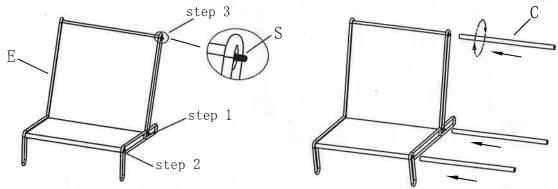
For easier assembly, We suggest assemble middle and front pole first, and then fix the screw for the backrest one.
