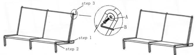
For easier assembly, We suggest assemble middle and front pole first, and then fix the screw for the backrest one.
